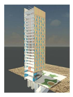
tilevered form necessitated unusually deep building piles and additional bracing. "Our structural design includes intricate links between the building frame and the foundation piles, along with a great deal of steel bracing for building support," Batt says. "All the building systems — the duct work, the sprinkler systems, the plumbing and waste lines — had to be woven through the structure."
